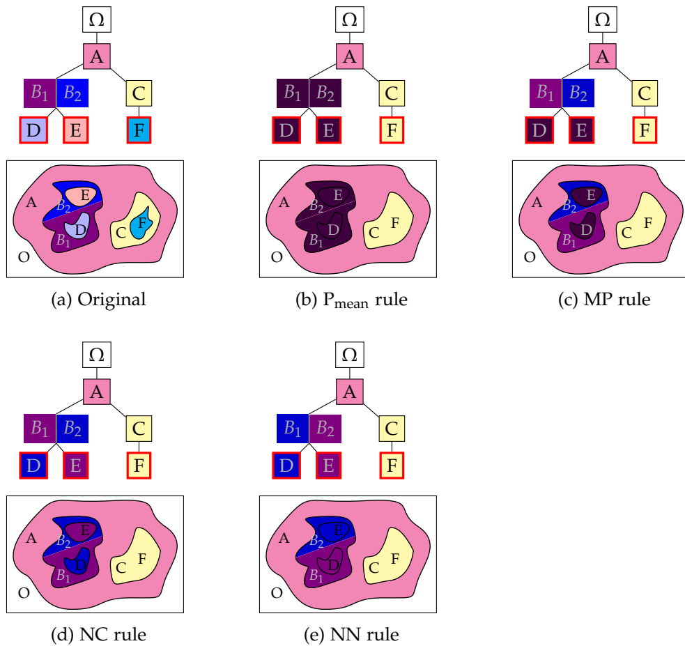
Figure 30: The different restitution strategies on the ToS when using a preorder on values. The nodes with red borders are those to filter.
