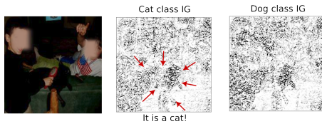
Figure 2: Attribution maps obtained by Integrated Gradients method. The pixels' importance is described from white to black (less to more important) according to a chosen class.
